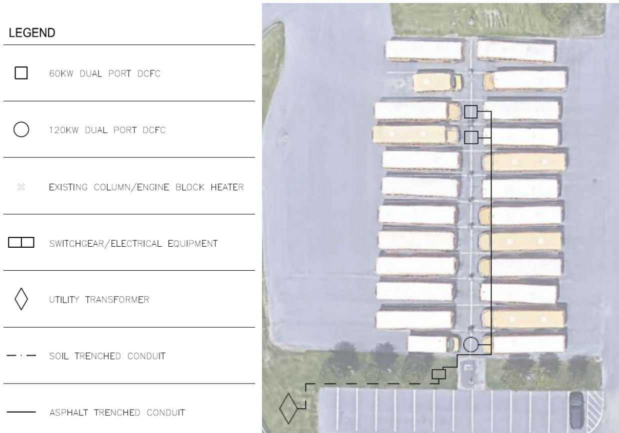
Figure 8: Phase 2 Installation Design
