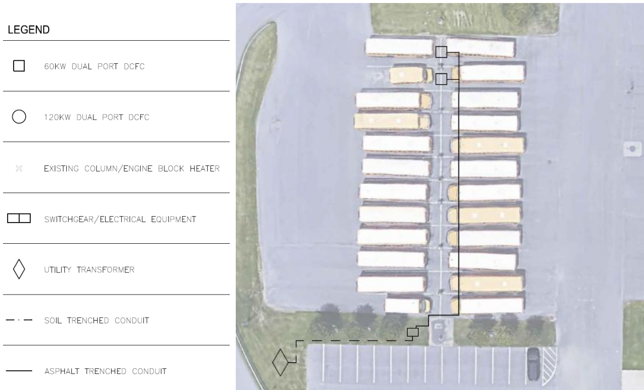
Figure 7: Phase 1 Installation Design
